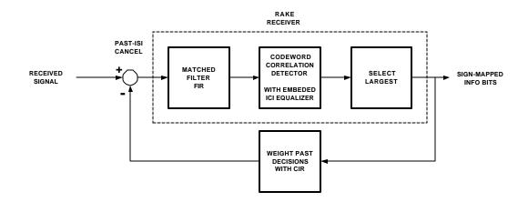
Figure 8. Rake receiver with ISI/ICI equalizer
