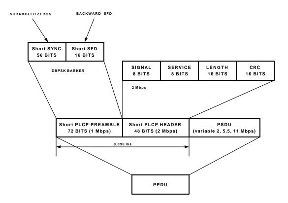
Figure 6. Short PLCP PPDU format.
