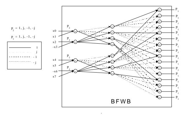
Figure 2. Basic Fast Walsh Transform Block (BFWB).
