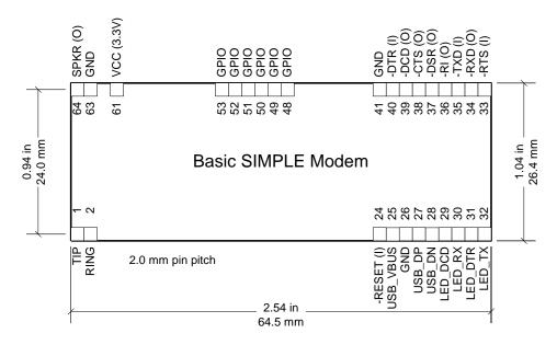
A VOCAL Augmented SIMPLE Modem (ASM) can be used as a stand-alone USB connected modem for various industrial applications. A built-in USB serial port recognized by Windows and Linux is used for full async modem operational control. One break-off leaf contains the isolated and protected telephone line interface. The other break-off leaf contains the USB serial port interface and 5V modem power supply.
