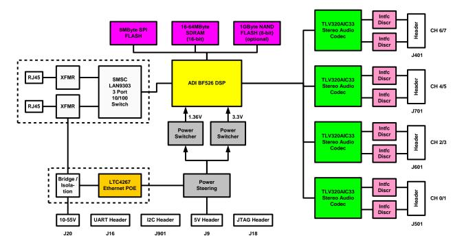
The four stereo audio codecs regarded as 8 audio channels are assigned to various analog inputs/outputs of the VAC as follows:
